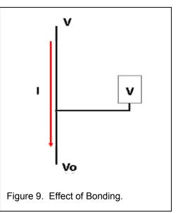
between those parts. In the figure, the electrical connection keeps the metal part at the same voltage as the conductor. (In actuality it will minimize the voltage difference.) This, in turn prevents or at least minimizes the electric field between the two as well preventing arcing. Since the metal part is 'floating' or not connected to ground, current does not flow through it. In some
