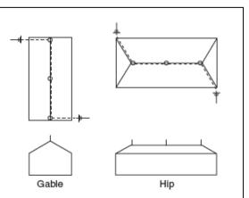
Figure 3. Example of Empirical Roof Rules for Gable and Hip Roofs. Circles denote air terminals, dashed lines denote conductors which terminate in grounding electrodes.
