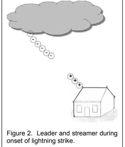
The upward and downward streamers are of opposite charge and are therefore attractive. When they
