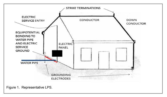
These subsystems function in a complimentary fashion to protect a structure from the damaging effects of lightning. Figure 1 illustrates a simple representative LPS that might be installed on a small structure. Each will be reviewed in turn and how they function will be discussed.
