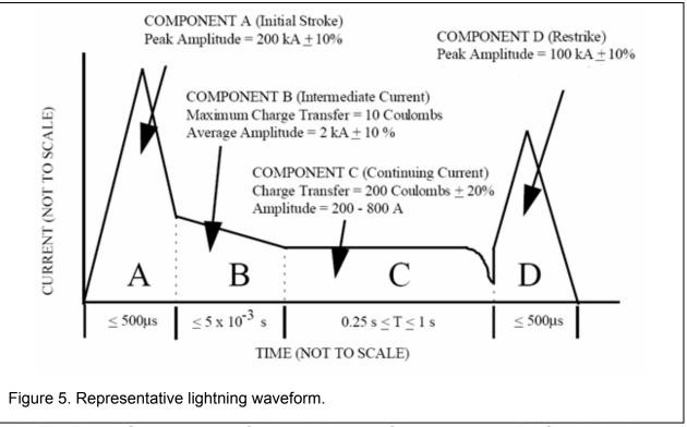
3) <u>The B and C components</u> of the lightning waveform are responsible for the heating and other ohmic effects on the conductor. Far more charge is transferred during the B and C components of the lightning event compared to the A and D components. While lightning
