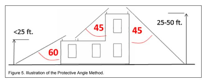
The protected angle method is also used with the empirical roof rules so lower attached may be protected. Detailed information to determine zones of protection are found in lightning protection design standards.
