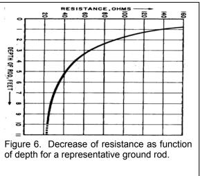
3) <u>Soil resistivity</u> is the single most important property that affects the final grounding resistance developed. In turn, several variables affect soil resistivity:
